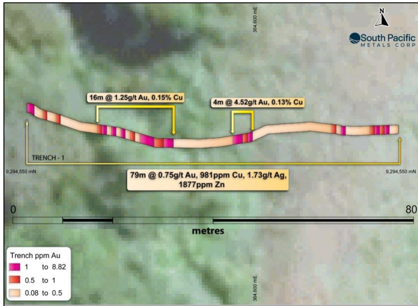
Figure 2: Ontenu Porphyry Prospect Trench 1 Gold Assay Results
