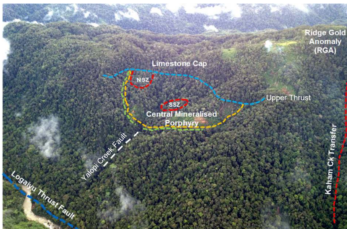
Figure 7-17: Oblique view of the Kili Teke prospect area (looking northeast) to show the location of the CMP (NSX and SSZ) relative to the Upper Thrust, the Logaiyu Thrust, and the Yalopi Creek and Kaham Creek Faults.
