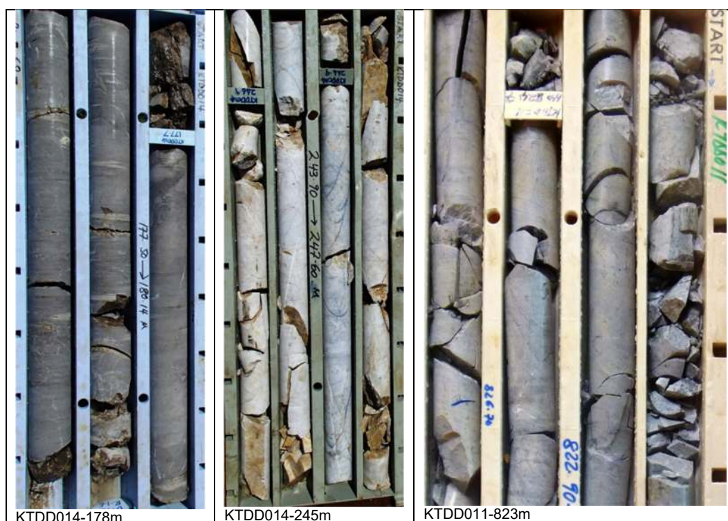
Figure 7-8: Examples of the host rock sequence – Ieru Formation siltstone, Darai Limestone and Marble.
