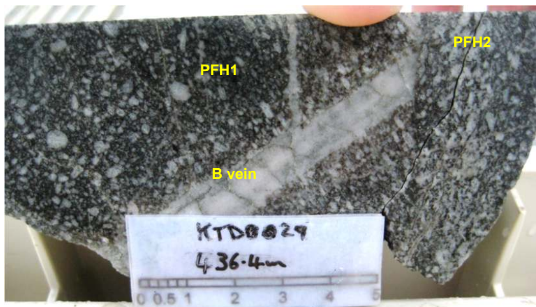
Feldspar Hornblende Porphyry (PFH1), with B type vein, cut by later Feldspar Hornblende Porphyry Phase (PFH2)
