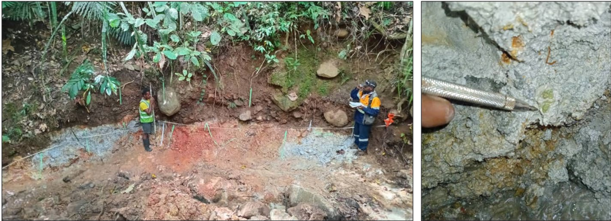
Figure 2: Newly identified Irinke Prospect Shear Zone exposed for mapping and sampling. Similarly styled host rock, alteration and sulfide mineralization as K92's Arakompa lode-gold vein, currently being drilled. Strong phyllic (sericite, quartz, pyrite) altered brecciated diorite exposed over 17 m length, 2 m width.
