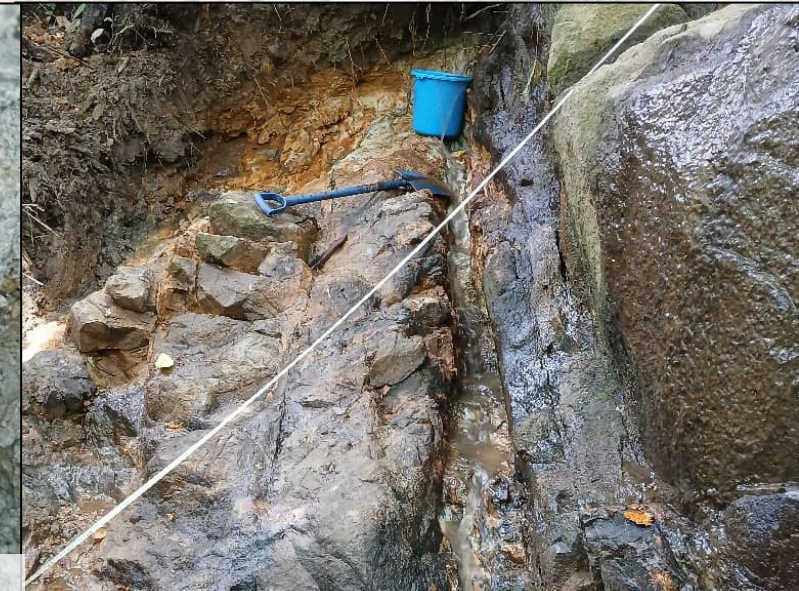
30 cm wide quartz-carbonate vein breccia that returned 2.28 g/t Au in 2022,
