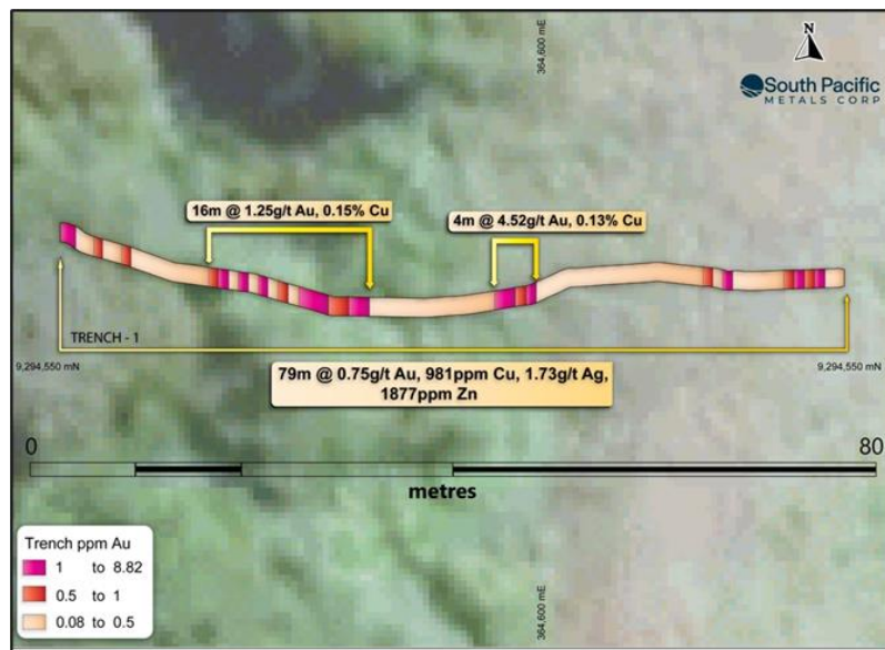
Figure 6 Trench 1 at Ontenu Cu-Au Prospect Gold and Copper Results
