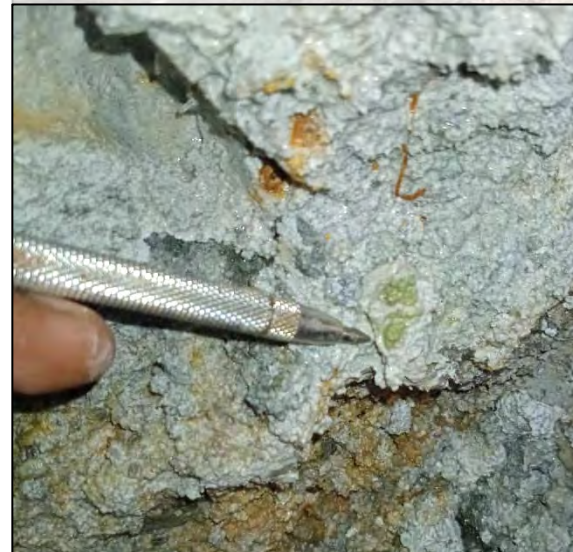
Chalcopyrite hosted in the strongly phyllic (sericite, quartz, pyrite) altered brecciated diorite.
